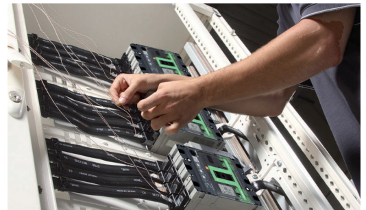
Temperature rise test in laboratory.
